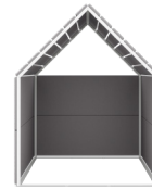
Gable semi open, roof panels
